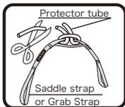
**1** Turn the emblem of the saddle strap (or Grab Strap) up, wind a protector tube around the upper side of the center of the saddle strap and cut the excess tube.
